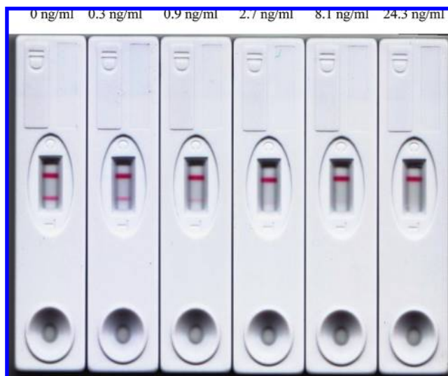
Figure 3. Standard ENR samples were tested using the test strips and the test lines with the naked eye.
